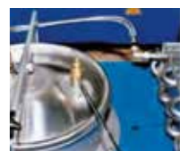
Safety valve in the container lid
